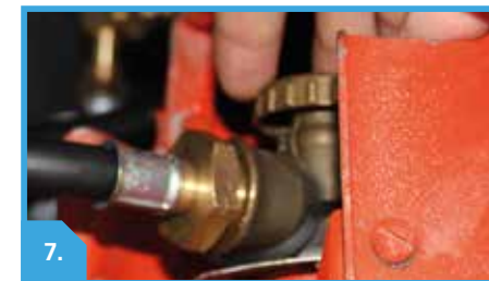
7. TURN OFF GAS BOTTLE VALVE WHEN PACKING DOWN
