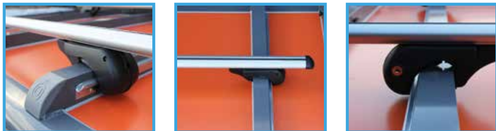
ROOF BAR FEET, CLAMP OVER THE GRIP RAILS FITTED ON THE ROOF LID RIBS.
