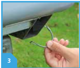
REMOVE THE D-PIN TO RELEASE LEG
